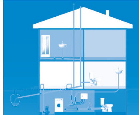
Figure 1: Example of installation with submersible pump:
